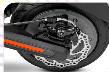
Brushless rear motor 500 W, 23.5 Nm, KERS, Peak Power 1500 W
