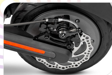
Motore Brushless 500 W, 23.5 Nm, KERS, Peak Power 1500 W
