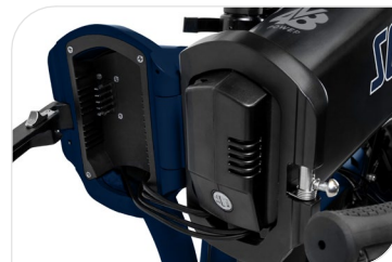
48 V, 10.4 Ah, 500 Wh Greenway battery, smart BMS, LG cells
