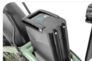
External battery 36 V, 10.4 Ah, 374 Wh, BMS
