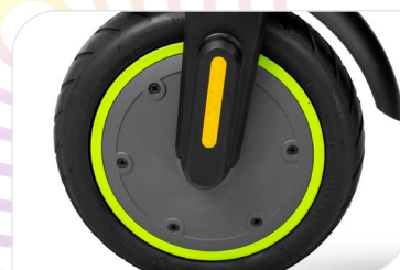
Brushless motor 250W, 14,5 Nm, KERS, Peak power 500W
