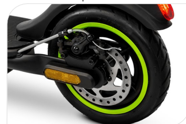
Front e-brake, rear disc, two levers
