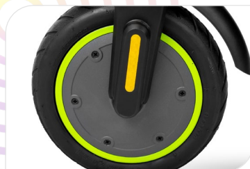
Motore Brushless 250W, 14,5 Nm, KERS, Peak power 500W
