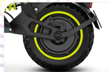
Motore Brushless 500 W, 22 Nm, KERS, Peak Power 3000 W
